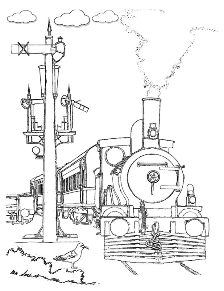
Locomotive C22 has just passed the lowered signal arm, this means it can keep travelling to the station. What do you think it means if the signal arm is raised? How are the signals operated?
